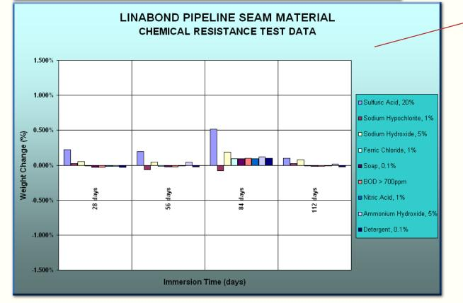
The tables to the left show the results of the chemical resistance tests which were conducted on the Linabond<sup>®</sup> Structural Polymer<sup>™</sup> Pipeline Seam Material, according to the <u>Standard Specifications for Public Construction</u> (Greenbook), Section 210-2; Requirements for Protective <u>Plastic Liners</u>. As you can see, the material far exceeds the requirements for constant immersion in wastewater, based on an expected 50 year design life.
